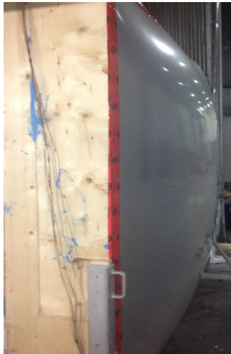
The test sample during the air leakage tests. (the sample was tested in the opposite direction after the first air leakage test cycle was complete)
