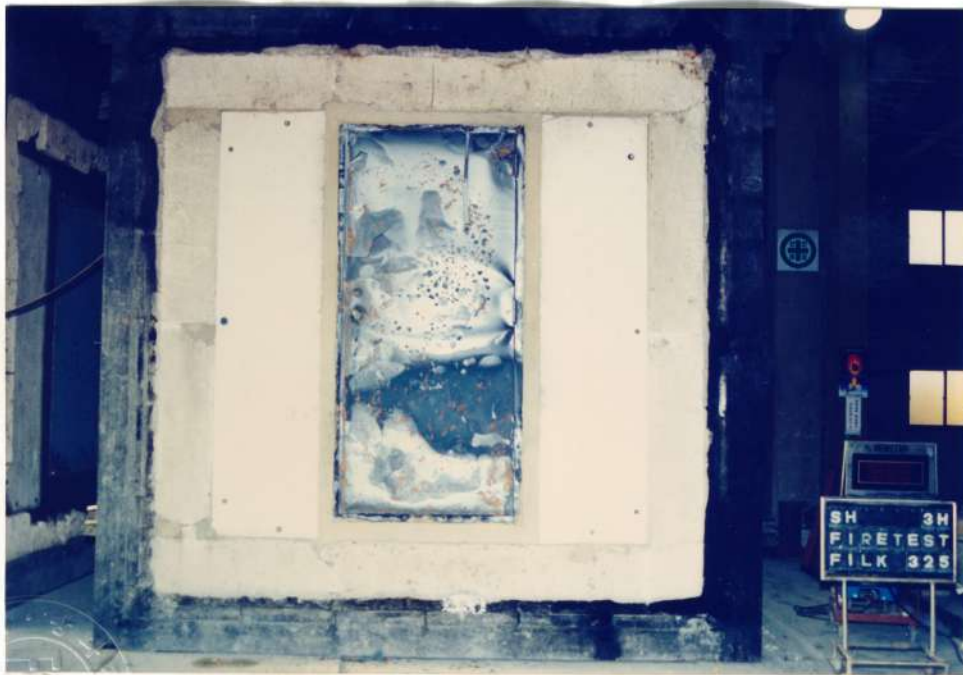
[Photo 6] The specimen after hose stream test
