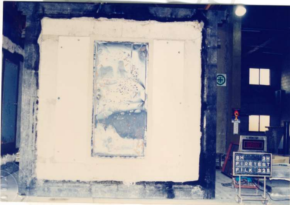
[Photo 2] Exposed face of the specimen after fire test.
