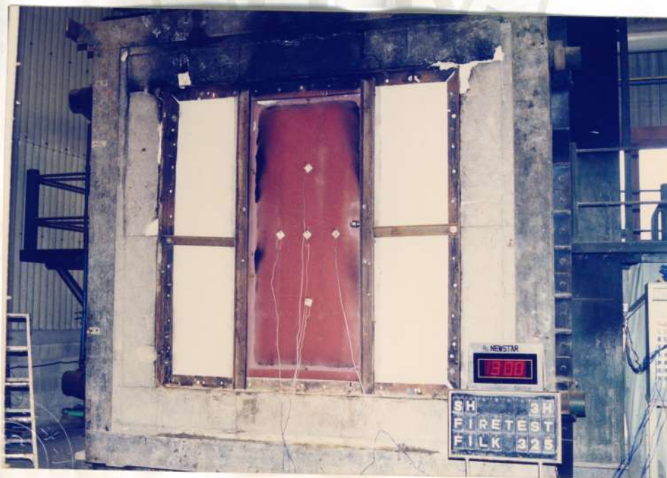
[Photo 4] Unexposed face of the specimen after fire test.
