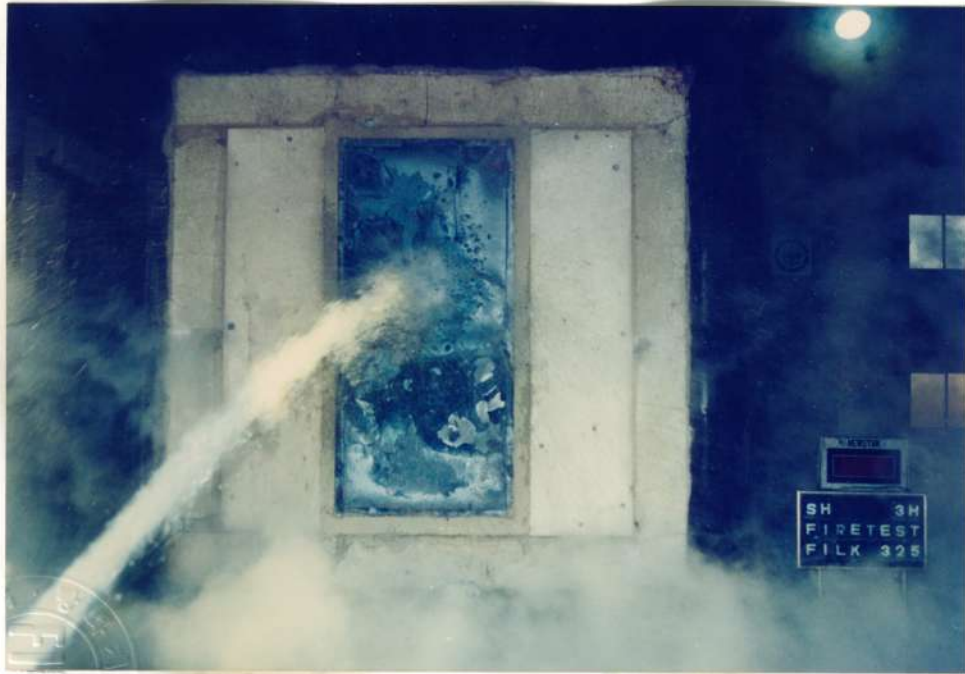
[Photo 5] View of hose stream test
