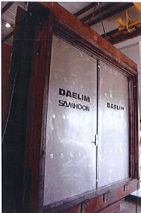
Pretest Photograph of Non-Loaded Side of Door
