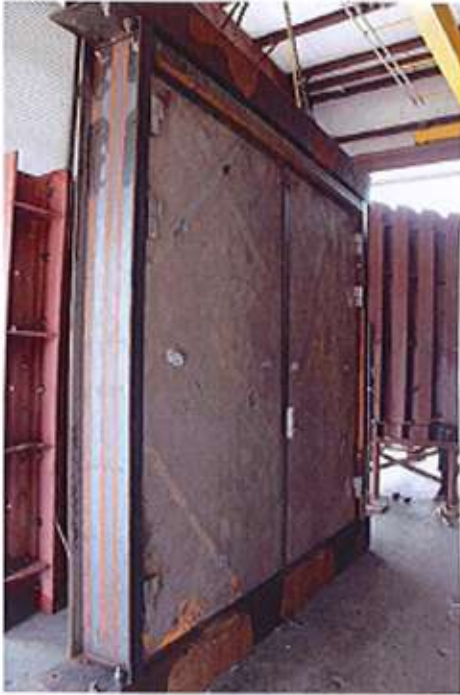
Pretest Photograph of Loaded Side of Door
