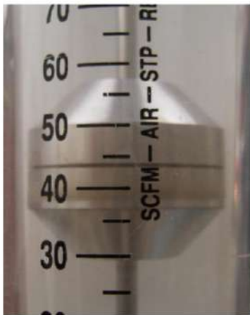
△ 44 cfm (AIR LEAKAGE @CHAMBER)
