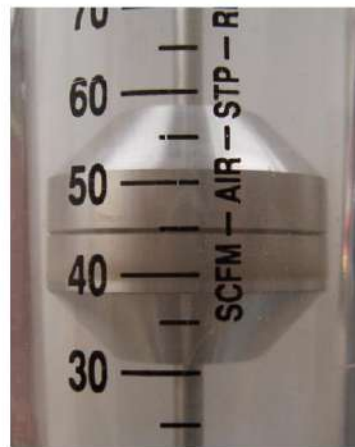
△ 45 cfm (AIR LEAKAGE @CHAMBER & SPECIMEN)
