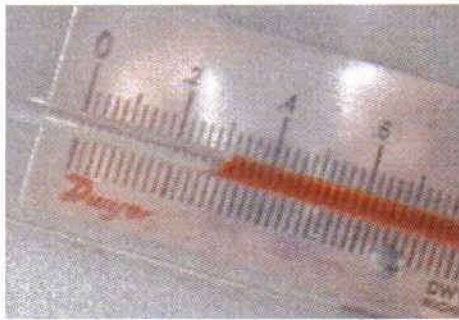
△ AIR PRESSURE DIFFERENCE 7.6 kg/m 2 (= 0.3"H 2 O)
