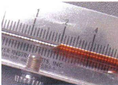
△ AIR PRESSURE DIFFERENCE 30.4 kg/m 2 (= 1.2"H 2 O)
